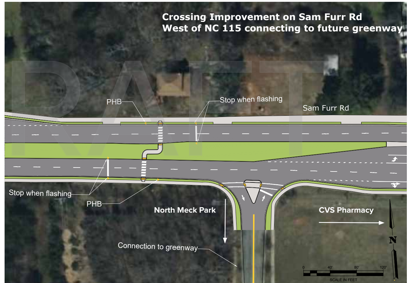
Figure 6.2. Conceptual design for crossing improvement to connect to North Mecklenburg Park and greenway.
